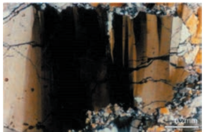
Figure 4. King band in olivine of Emir Abdelkader peridotite block. Figura 4. Kink bands en olivino en la peridotita.
